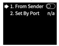
In the submenu, press the knob/**OK** to set the sender as the connection source. Then select **Set By Port** to enter the submenu, in which you can choose the Ethernet port that needs setting mapping, and set the offset values of X and Y, and the width, height, row number, column number and link type of the corresponding cabinets. Finally select **Save** to save the mapping.
