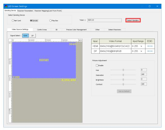
Click Detect Receivers. On the Detect Receivers sub-page, click Detect All Receivers, and the software will automatically acquire information such as the port, index, running time, and supported chips of the receiver card. Please check the corresponding cable if
