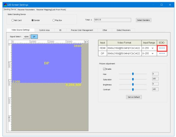
In the **Resolution (EDID) Setting** dialog box, the resolution of the current sender is displayed by default. Click the dropdown button. From the resolution list, you can select a conventional resolution, or select **Custom** and set the width, height, frame rate and standard of the customized resolution.
