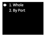
Output shift contains two selections: Whole and By Port. On the submenu of Whole, you can rotate the knob to set the row starting point (X) and the column starting point (Y) of the whole image and then save the setting; on the submenu of By Port, you can respectively set the row starting point (X) and the column starting point (Y) of the image of the 20 Ethernet ports, and then save the setting.
