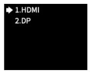
In the EDID setting submenu of **HDMI** or **DP**, you can rotate the knob and select a conventional resolution to save the selected resolution to the sender, or select **Custom** and set the width, height and frame rate, and then select **Save** to save the setting to the sender.
